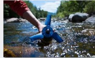
Conventional Axial Flow Lift based Turbine for Tidal Current (Left) and an Estream @ miniature Turbine in a River (Right)
