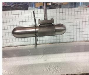
Fig. 3 horizontal axis free-stream turbine
