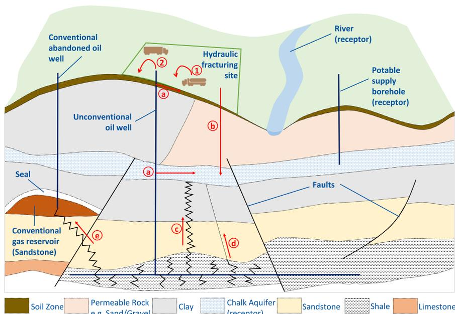
Fig. 1 A conceptual model indicating the main potential contaminant pathways reaching groundwater from a hydraulic fracturing site. The letters correspond to individual contaminant pathways: a) well casing failure, b) infiltration, c) fracture propagation, d) natural fracture connection, e) connection with old oil wells. The numbers correspond to spills on site: 1) chemicals spills, 2) returned flowback/produced water spills from wells.
